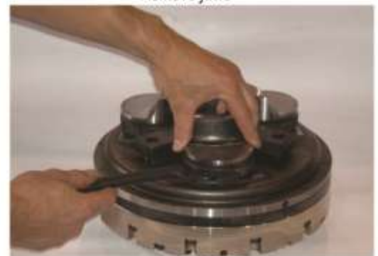
Install jaw and tighten
