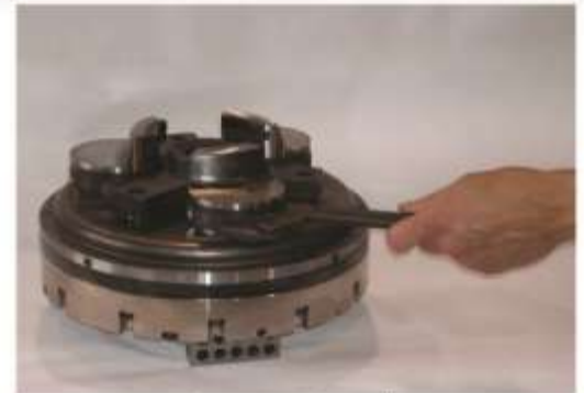
Loosen retention coupling
